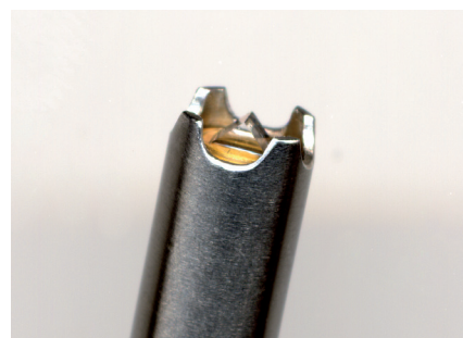
IN350-T Diamond ATR Probe head.
