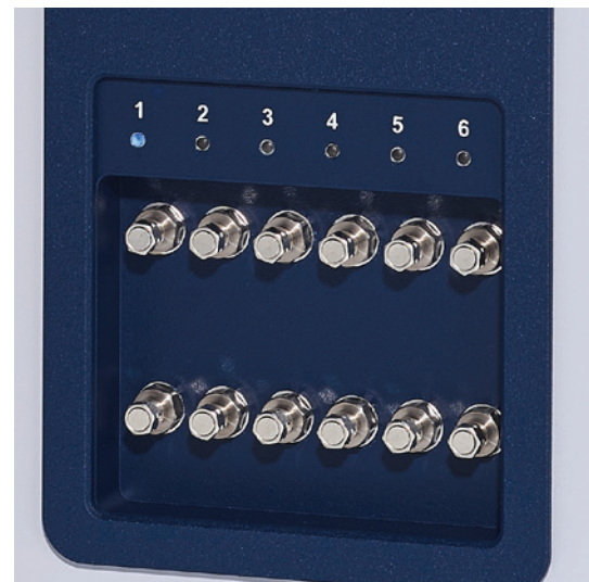
Internal 6-port multiplexer
