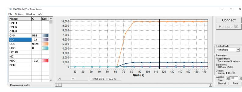
Software package OPUS GA for automated identification and quantification of gas compounds. The time series window displays the concentration of selected gas compounds in a gas mixture as a function of time.
