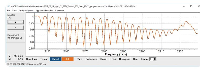
Measurement (blue) and fit (orange) to quantify the amount of carbon monoxide. Also, the contributions of the interfering carbon dioxide and nitrous oxide are considered in the fitting routine such that the measurement and the result of the fitting procedure show an excellent agreement.
