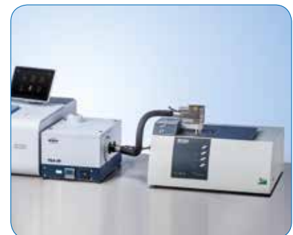
Various external accessories, such as the TGA module, can be coupled to INVENIO.
